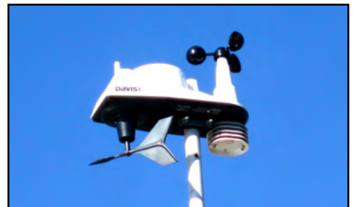
Stroud's weather station runs on a small solar panel and transmits data by radio.
